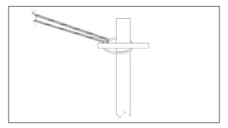
The 12/20 pegs must be hammered all the way down, so the horizontal part of the peg secures the flysheet to the ground.
