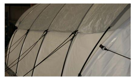
Place the flysheet with the 6 poles inserted on top of the tent roof.
