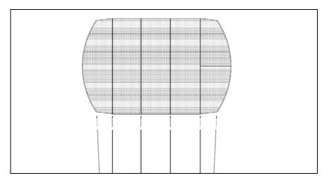
Push the poles through the channels of the flysheet, enabling the poles to reach equal distance out from the flysheet.
